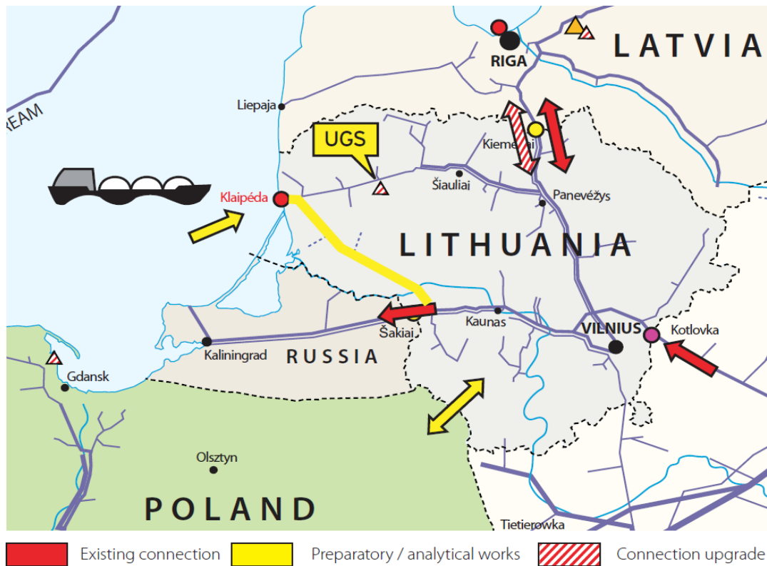
Figure 1.4.3 Infrastructure of natural gas in Lithuania 38
