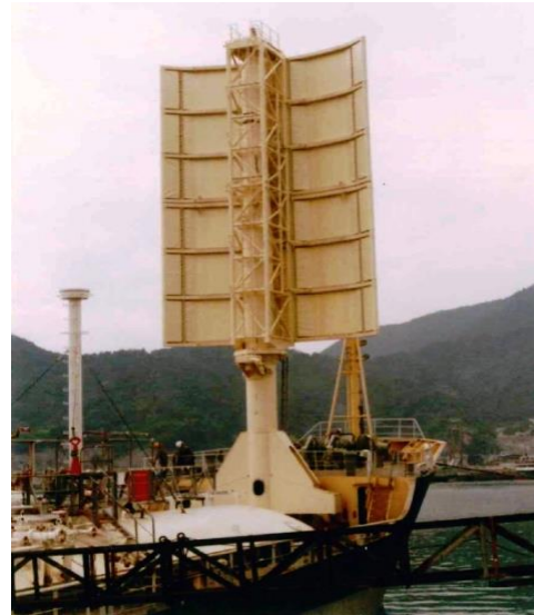
Figure 3: JAMDA Rigid Sail at Teramoto Iron Works in the 1980's, Eco Marine Power
