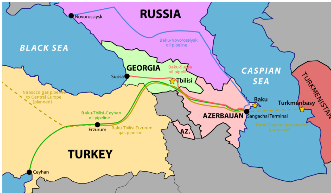
Picture 10: Pipelines from Sangachai Terminal, source: https://en.wikipedia.org
